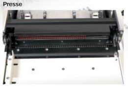
Only 1 variable closing unit needed for all book thicknesses. The change-over time of the closing unit to the according diameter is done in a few minutes.
