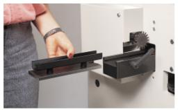
For each diameter an according two-divided feeding channel is used. Easy and fast change by release of two clamping screws.
